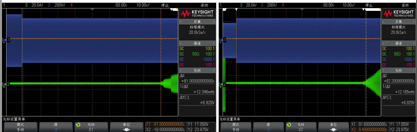
Re-connection after voltage fault
